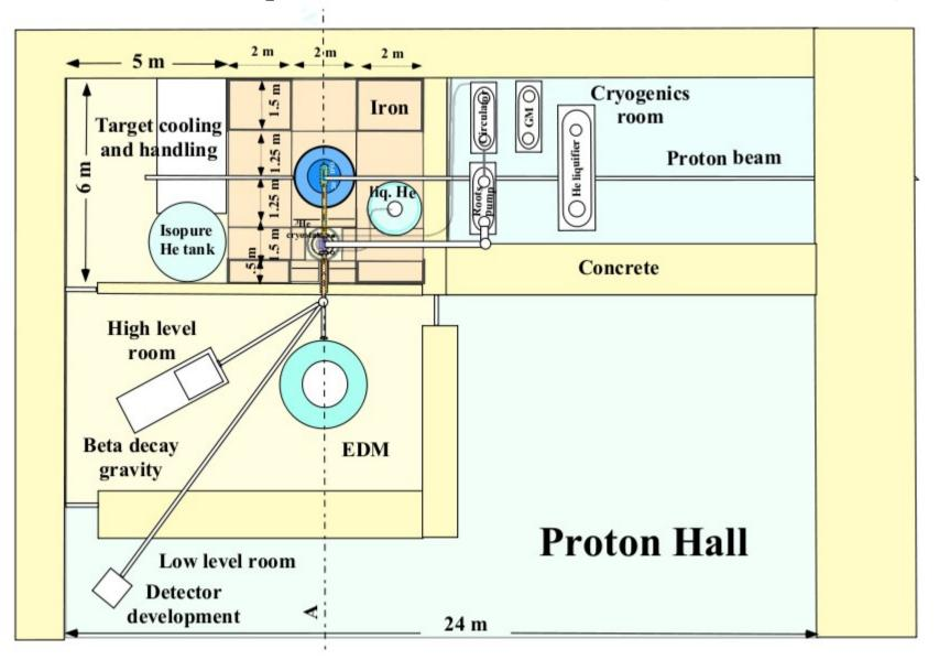
layout still needs some work... cryogenics location, shielding, remote handling
