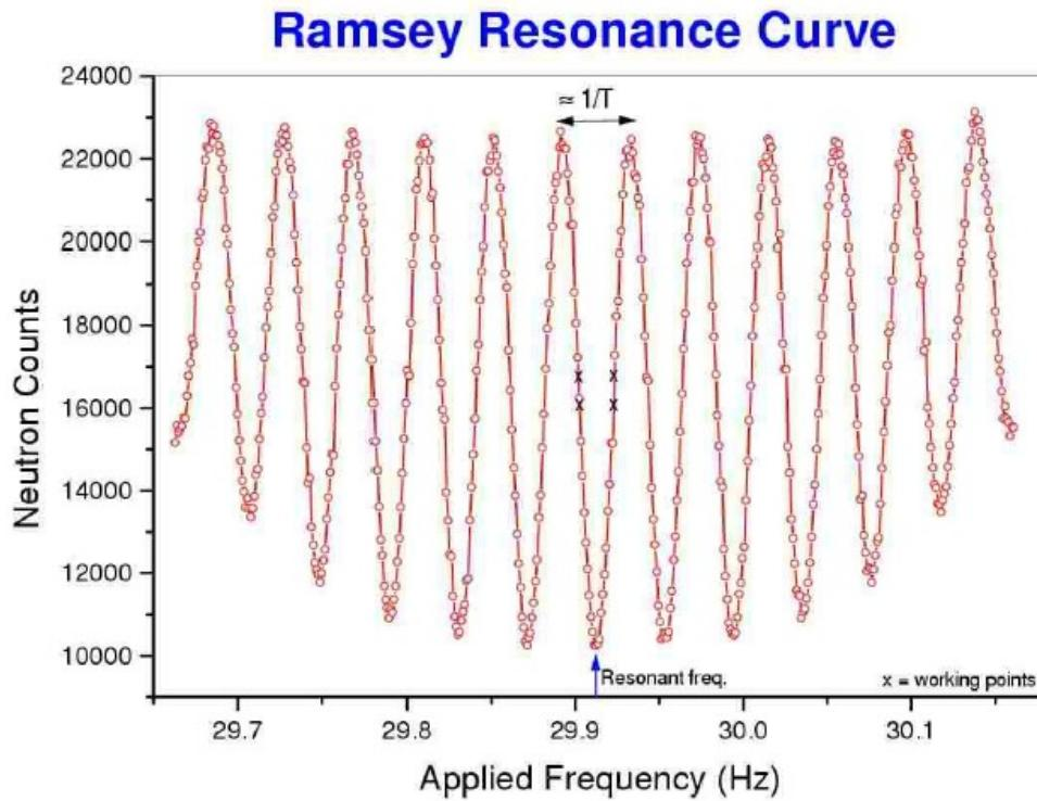
Sit at the steepest slope and watch for any change in neutron counts under E-field reversal.
