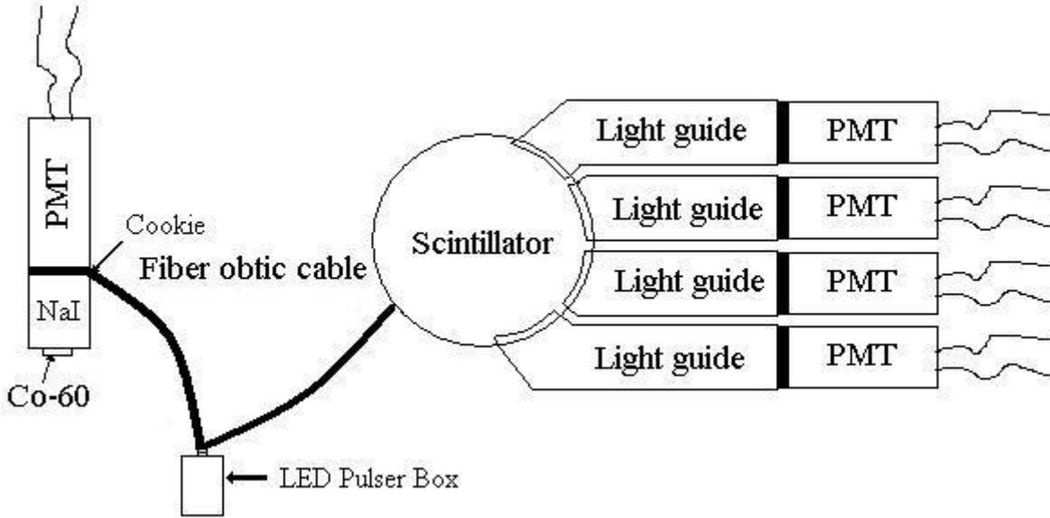
Figure 1: Setup Schematic
