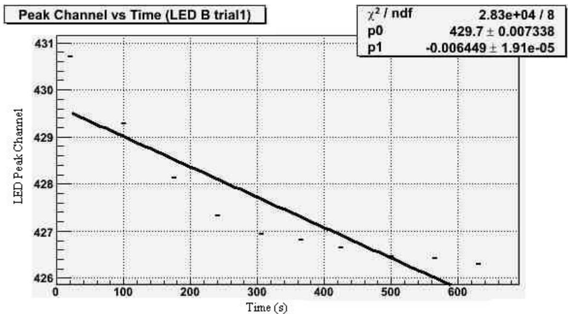
Figure 12: LED peak vs time. Drift test 1, LED B
