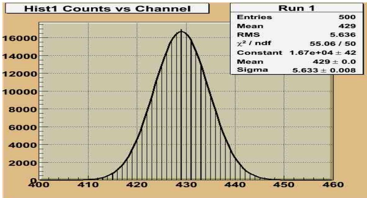
Figure 7: Typical pulse height spectrum fit with a gaussian (LEDBtrial2run1)
