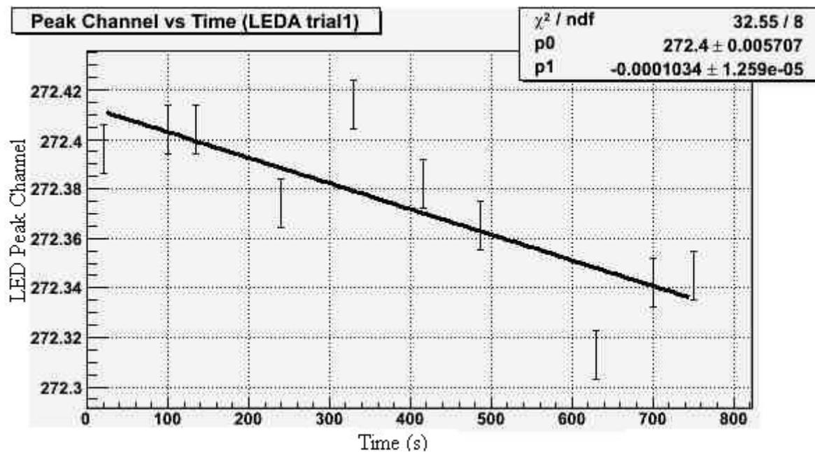
Figure 10: LED peak vs time. Drift test 1, LED A
