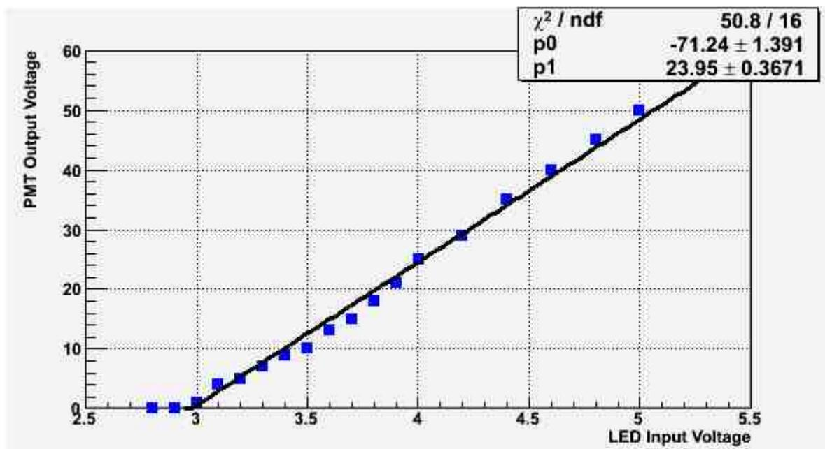
Figure 8: PMT output pulse heights dependance on LED input voltage
