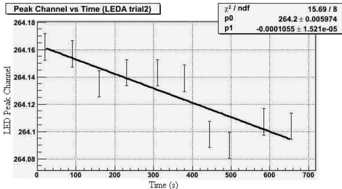
Figure 11: LED peak vs time. Drift test 2, LED A
