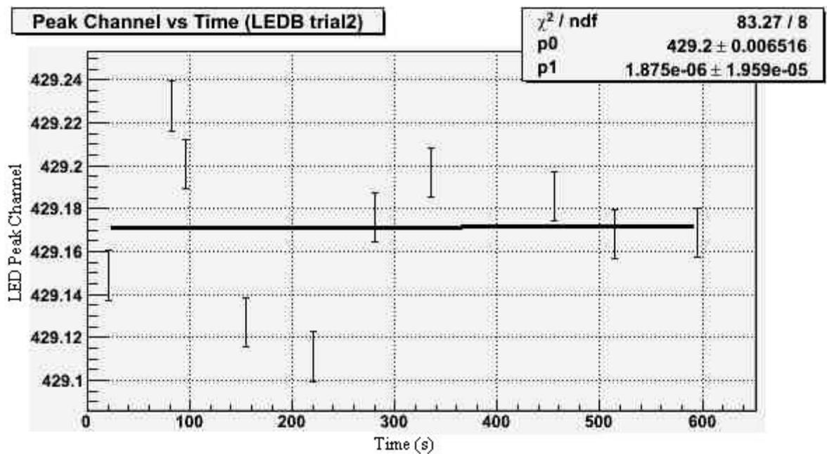
Figure 13: LED peak vs time. Drift test 2, LED B
