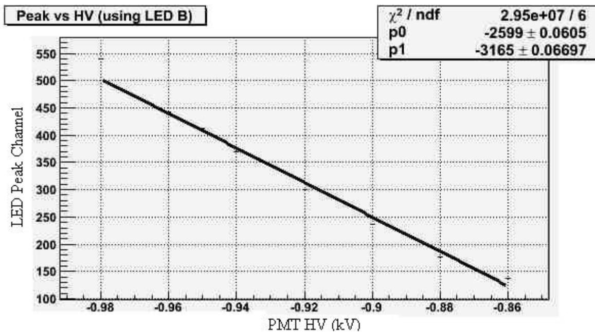
Figure 9: LED peak vs PMT HV is a linear
