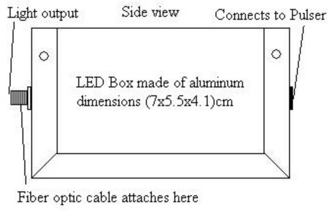
Figure 5: Diagram of LED Box constructed for UCNA
