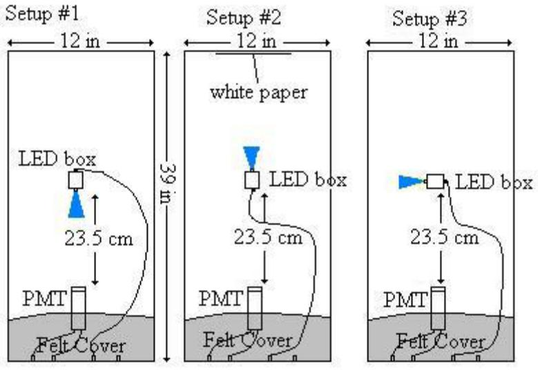
Figure 4: Setups 1,2 and 3, Setup #1 saturated the PMT, Setup #3 was used for all reported tests
