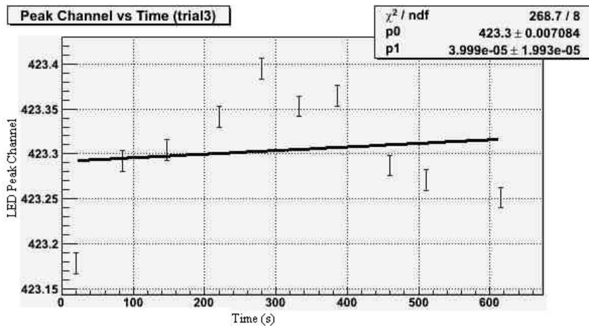
Figure 14: LED peak vs time. Drift test 3, LED B
