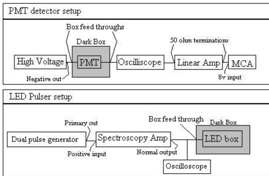
Figure 3: **Block diagrams for the LED drift experimental setup**
