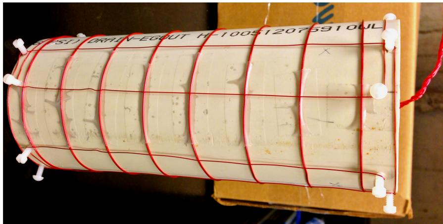
Figure 3.5: Coil for the new magnetic shield. Off axis field coils wound parallel to the centre axis of the tube.
