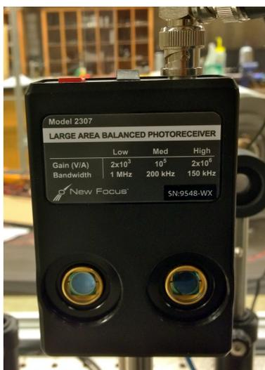
(c) New Focus dual photodiode
