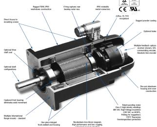
Danaher DC servomotor with NEMA 34 mount,
