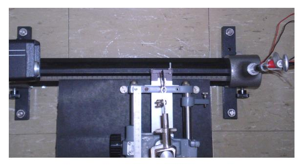
blocking arm simulates the scanner, moving between the laser and photodiode.
