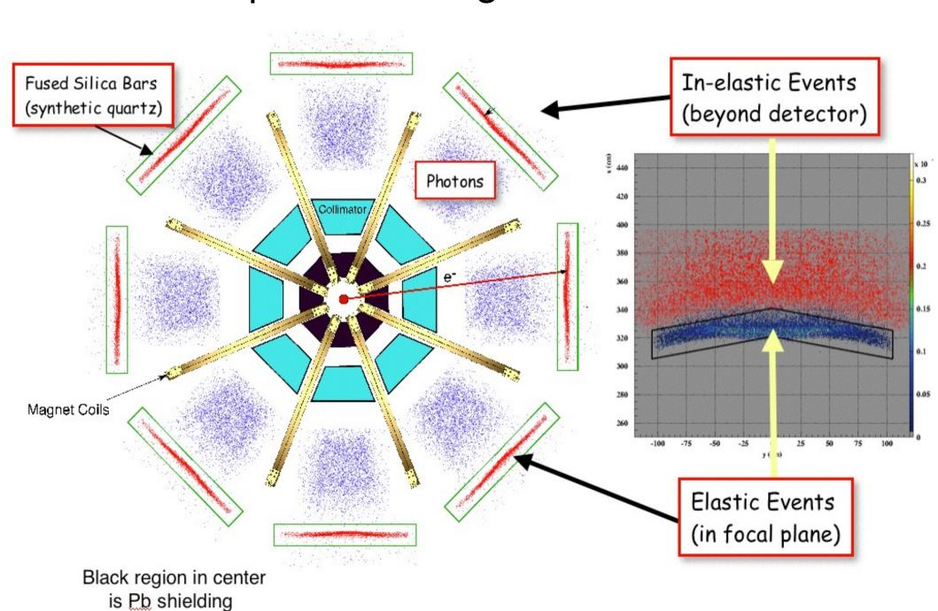
Production Mode: Actual asymmetry measurement 180  $\mu A$  electron beam, high detector rate, current mode readout
