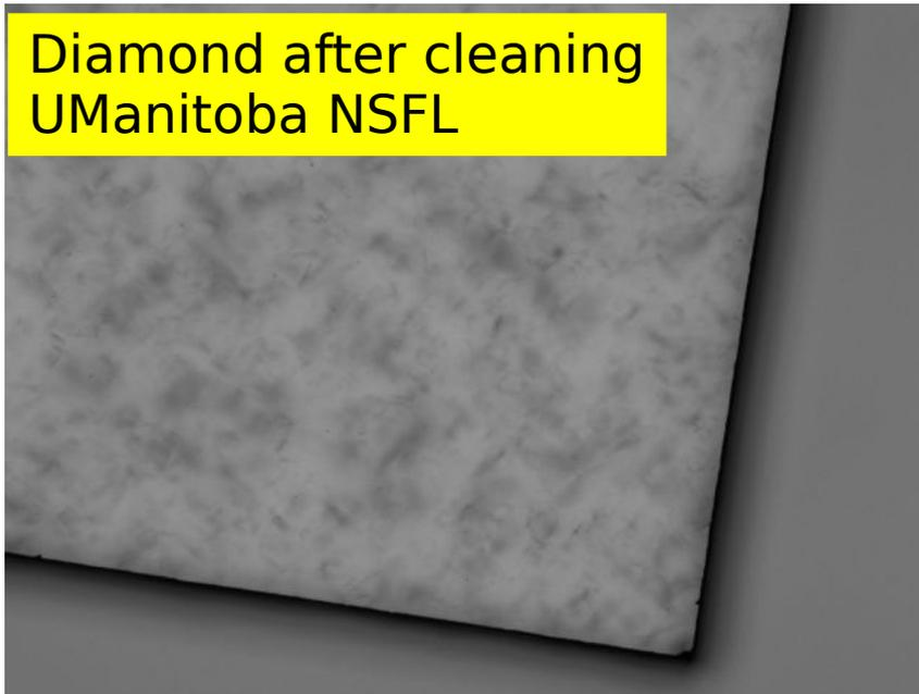
We use pc-CVD (polycrystalline chemical vapour deposition) diamond from Element Six, UK.
