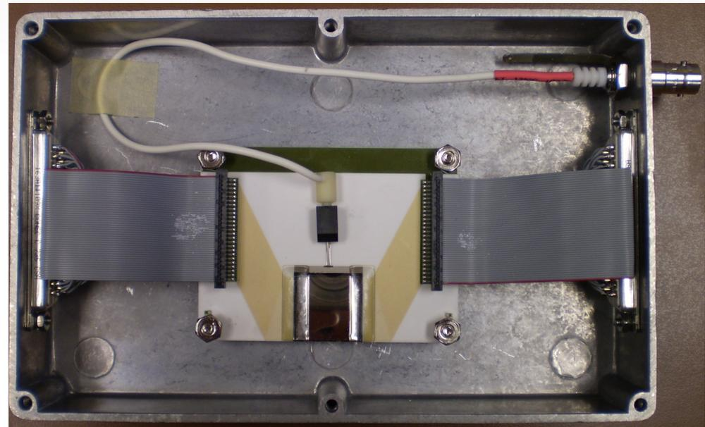
Test setup for radioactive sources
